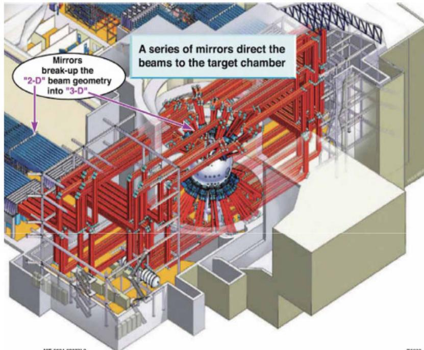
NIF Laser System: 192 laser beams
