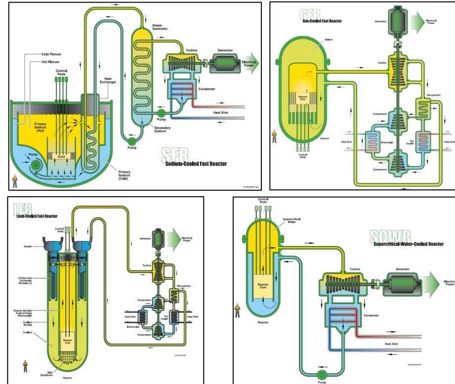
→ **fast neutron** induced fission is used to produce electrical power and to burn up long lived actinides
