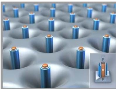
Picture: While transistors have been arranged on a flat plane so far memory chips based on nanowires protrude from the chip. This concept could revolutionize the architecture of chips.
