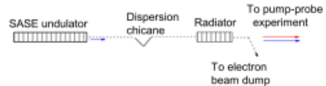
FIG. 1. (Color) Scheme of the afterburner for pump-probe experiments at an x-ray FEL.
