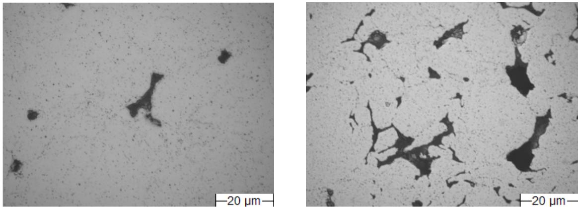
Fig. 3: Polished sections for ODS0.3Al10 (left) and FeCr20 (right)
