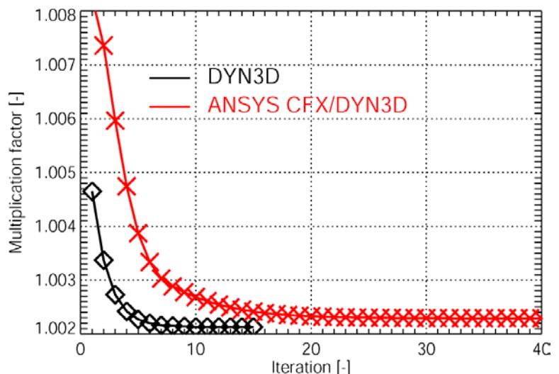
Fig. 2: Convergence of steady-state calculations
