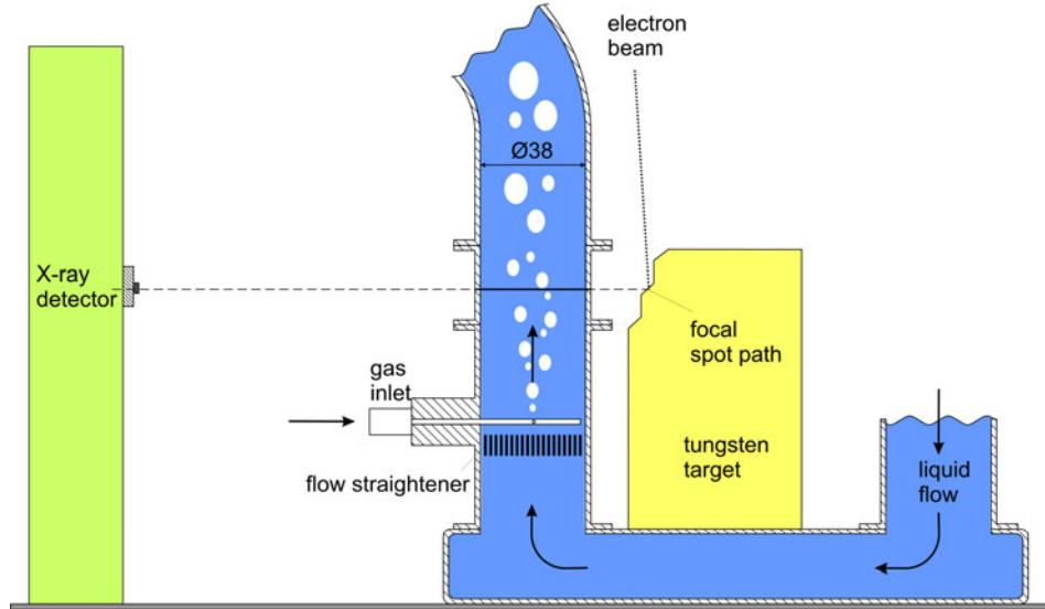
Fig. 2: Experimental two-phase flow loop setup
