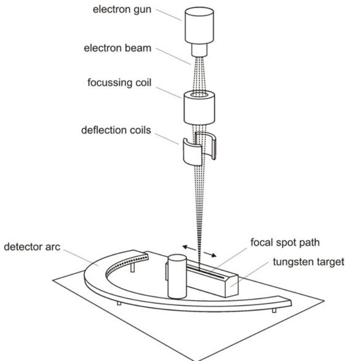
*Fig. 1: Principle of ultrafast electron beam X-ray CT*
