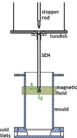
*Fig. 4: Detailed view on tundish with stopper rod, SEN and mould*
