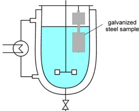
Fig. 2: Experimental set-up for batch studies
