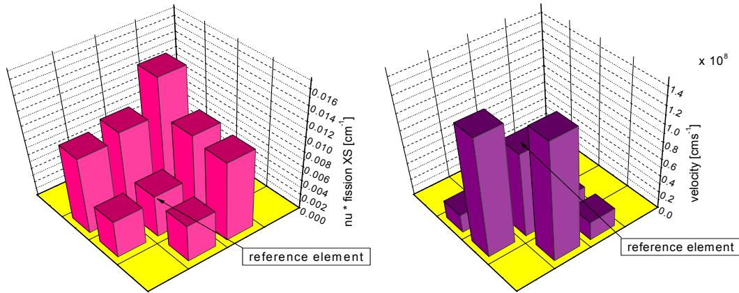
Fig. 4: Neutron production cross section (left) and neutron velocity (right) for the different fuel elements and areas in the fast part of YALINA-booster for SC3B
