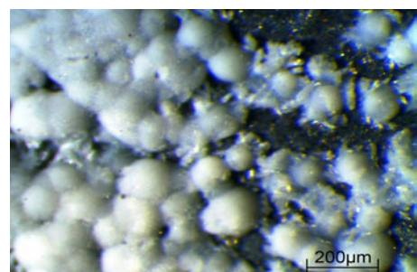
Fig. 7: Zinc borate on a sample
