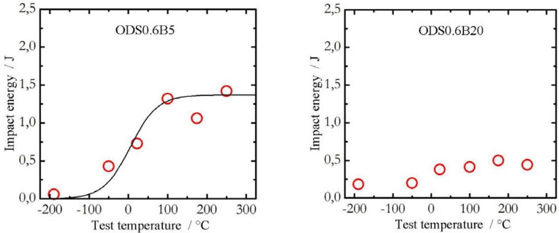
Fig. 4: Impact energy versus test temperature for ODS0.6B5 (left) and ODS0.6B20 (right)
