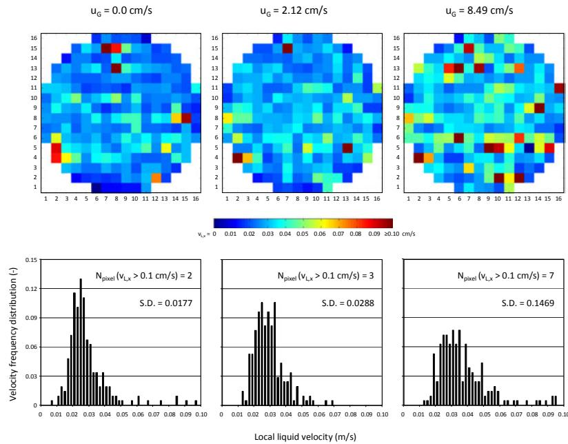
Fig. 4: Effect of superficial gas velocity on liquid velocity distribution and corresponding frequency distribution of the local liquid velocities ( $u_L = 0.71 \text{ cm/s}$ )
