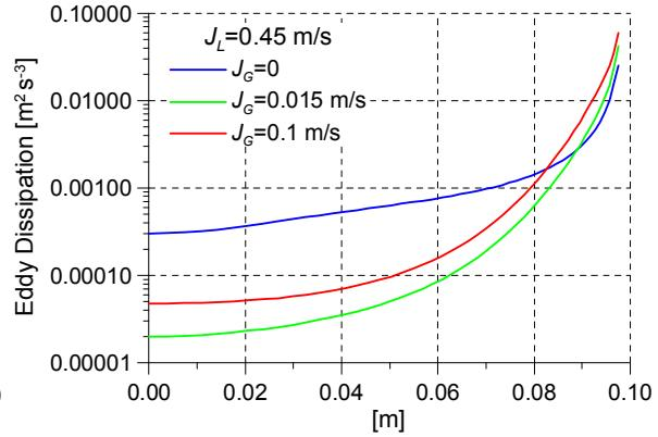
Fig. 2: Calculated profiles for the eddy dissipation
