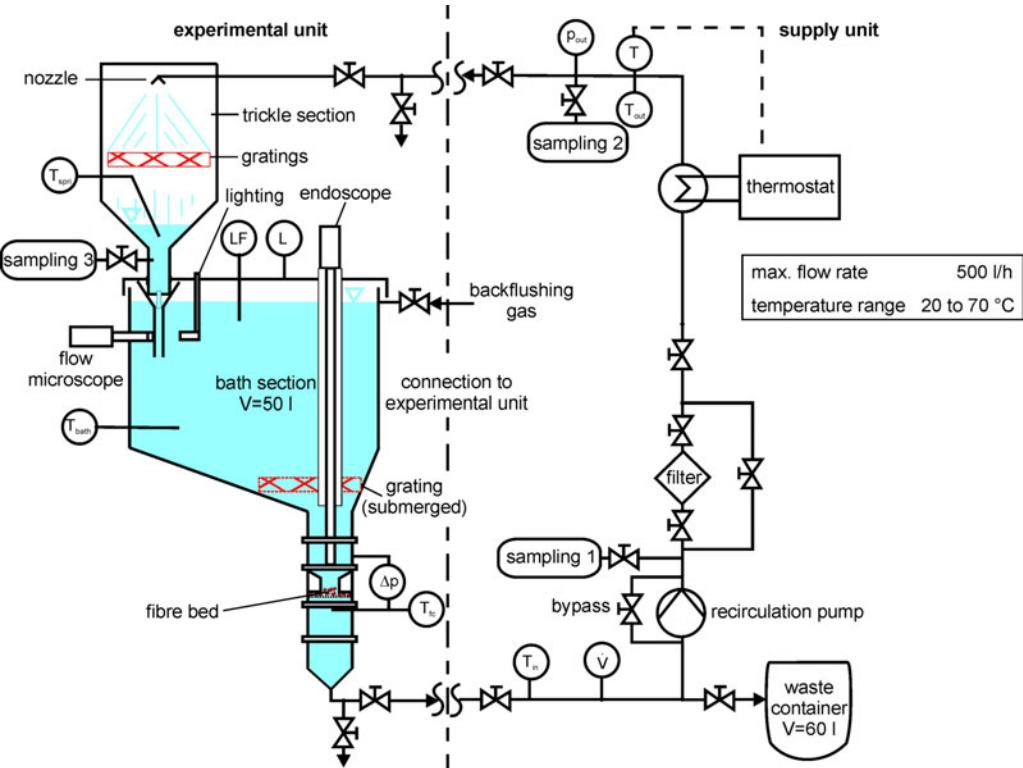
Fig. 4: Experimental set-up for long-term corrosion experiments
