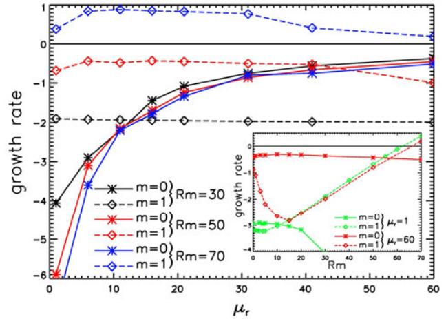
Fig. 6: Growth rates of the field amplitude (without  $\alpha$ -effect). Solid curves represent the results for the axisymmetric mode ( $m=0$ ) and dashed curves show the ( $m=1$ )-mode. The inset plot presents the growth rates for  $\mu_r=1$  and  $\mu_r=60$  in dependence on  $Rm$ .
