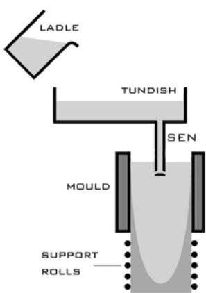
Fig. 1: Principle of the continuous casting process
