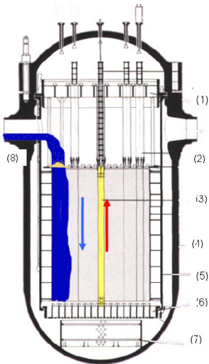
Fig. 1: RPV with ECC injection
