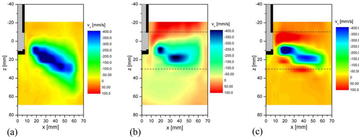
*Fig. 5: Time-averaged, horizontal flow at the nozzle outlet (a) without magnetic field, (b)  $B = 310$  mT, non-conducting channel (c)  $B = 310$  mT, conducting channel*
