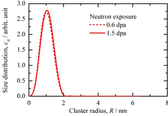
Fig. 3: Particle volume size distribution functions of irradiation-induced scatterers
