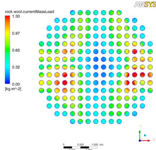
*Fig. 4: Rock wool mass load [kg/m<sup>2</sup>]
