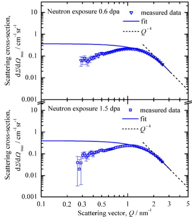
Fig. 2: Difference nuclear scattering cross sections for Fe-12.5at%Cr irradiated up to 0.6 and 1.5 dpa with the unirradiated control taken as reference
