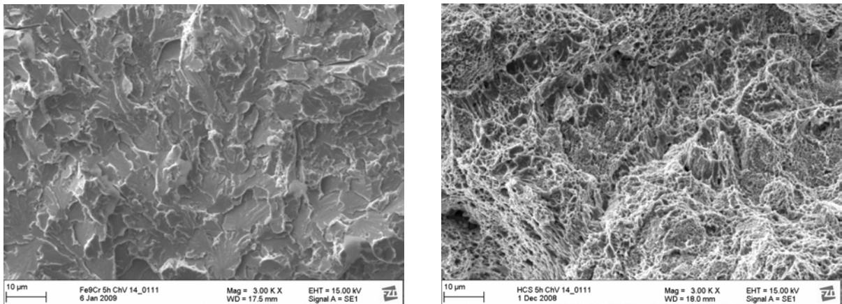
Fig. 5: Fracture appearance for FeCr5 tested at -190°C (left) and ODS0.3A5 tested at 175°C
