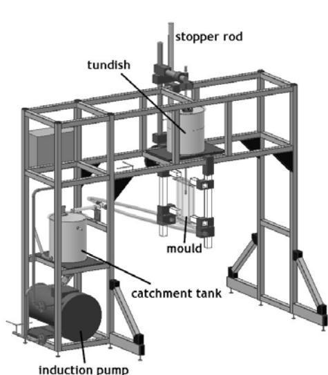
*Fig. 3: Schematic view of the Mini-LIMMCAST facility*
