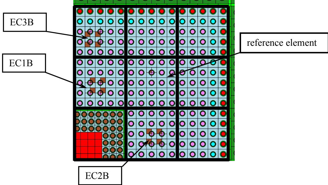
Fig. 1: Central fast area of the YALINA-booster core
