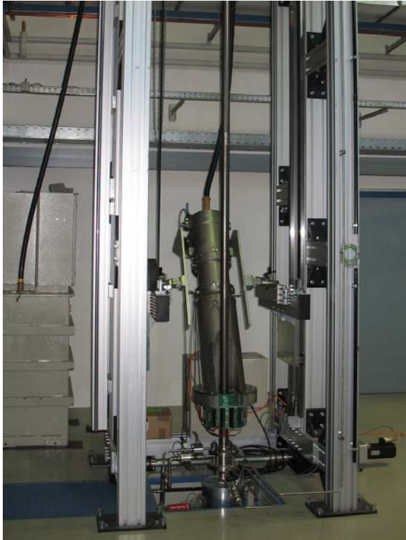
Fig. 3: Scanner mounted at a vertical test section at FZD's TOPFLOW facility
