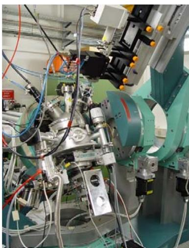
Fig. 1.: Sputter deposition chamber.
