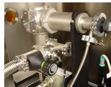
**Closed-cycle He cryostat** with large fluorescence window adapted to the 13-element detector and very low vibration levels cools samples down to 15 K.
