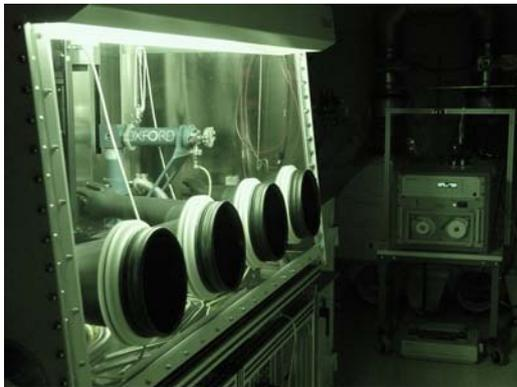
During the measurement, the **spectroscopic glove box** envelops the samples, which are mounted either on a remote-control 8-fold multistage holder or in a cryostat. The fluorescence and transmission detectors remain outside of the glove box.
