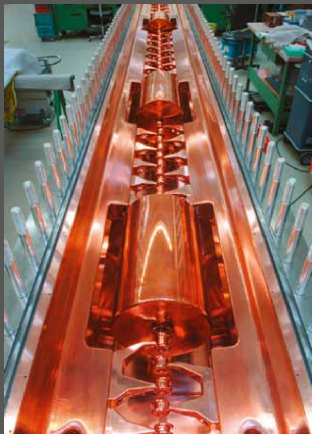
Inside view of the GSI-developed five-meter-long linear accelerator for the Heidelberg Ion-Beam Therapy Center. Image credit: GSI Helmholtz Centre for Heavy Ion Research/G. Otto
