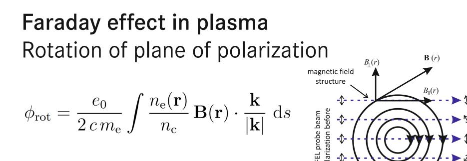
Simulations show magnetic fields up to 10 kT with radial dimensions of about 5  $\mu$ m.
