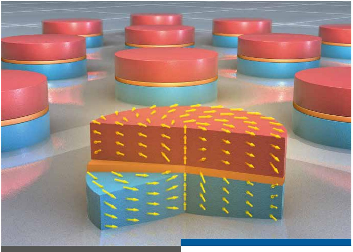
**STABILITY THROUGH A VORTEX:** Within the space between two magnetic layers, static three-dimensional magnetic vortices form around a non-magnetic intermediate layer. They act to stabilize the direction of magnetization in the vortex' central core – a prerequisite for the kind of stable vortex antennae applicable in wireless data transfer. Diagram: Sander Münster
