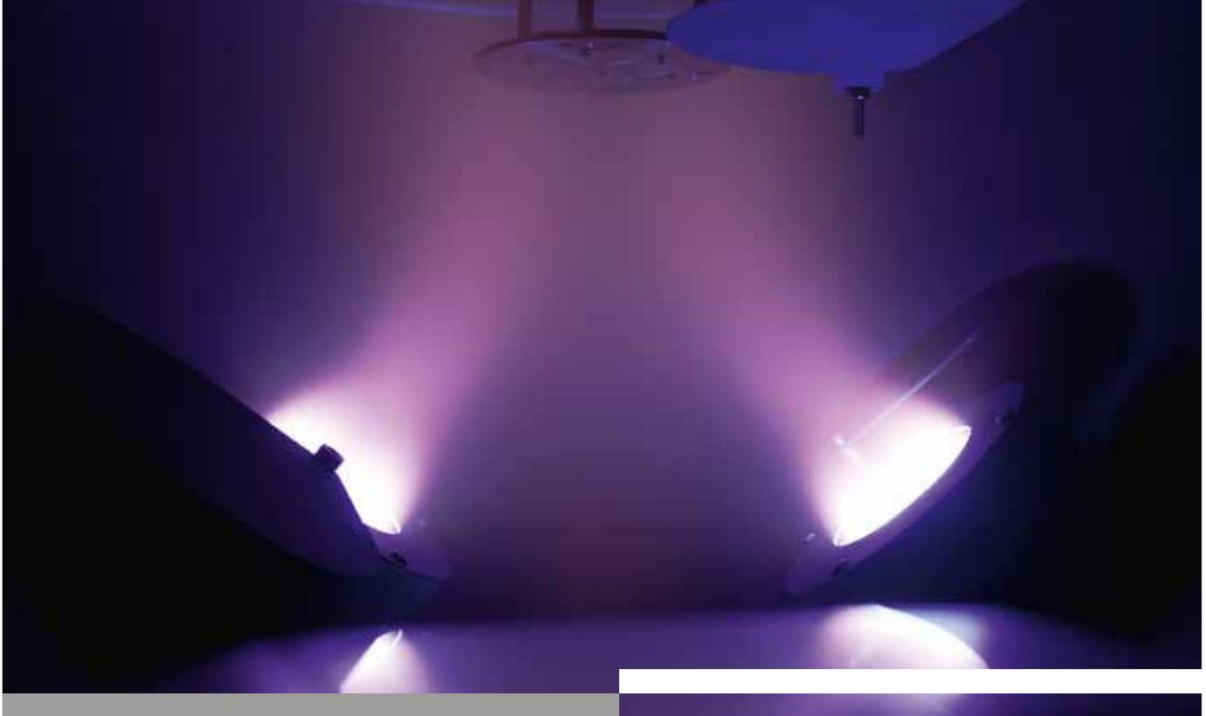
**GASEOUS DISCHARGE:** Whereas a fluorescent lamp's gas or glow discharge is what makes it light up, its job inside this coating chamber is to ionize argon atoms that emit a purple glow.
