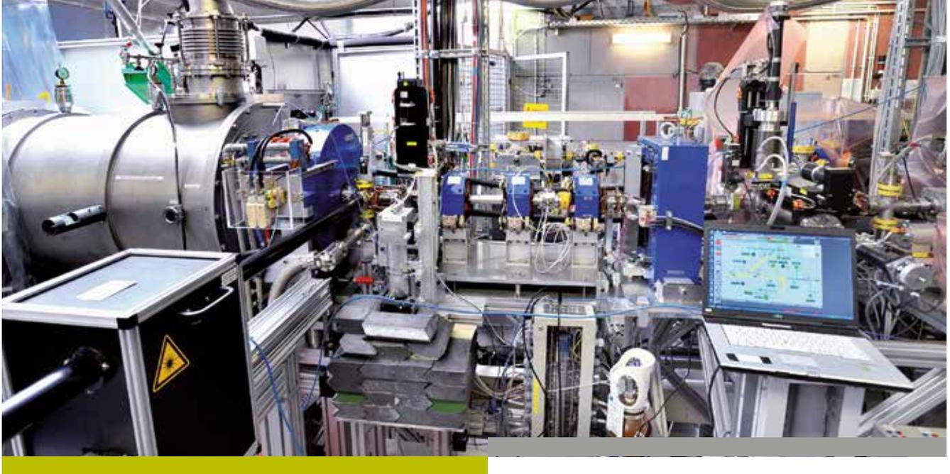
**SOURCE OF RADIATION:** Gamma rays used in the study of atomic nuclei are produced when fast-moving electrons from the ELBE accelerator hit a special target. This strongly decelerates the electrons, which is why physicists speak of "bremsstrahlung."
