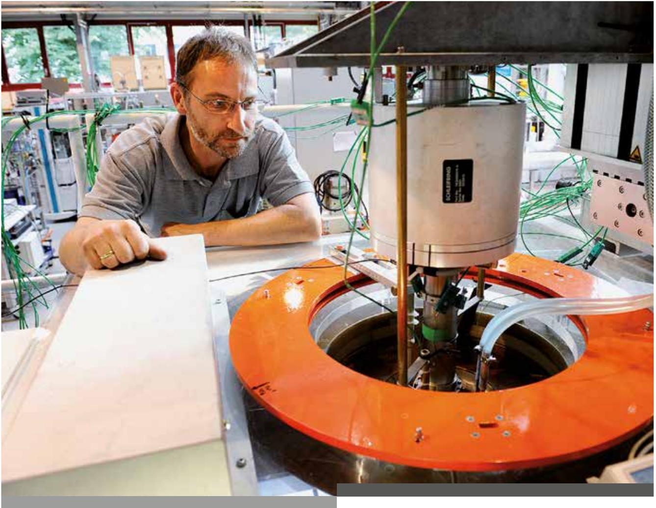
**WITHOUT A SINGLE TOUCH:** Magnetic fields stir liquid metals but they are also capable of flow deceleration and acceleration. Josef Pal is seen here conducting an experiment at the HZDR's MULTIMAG (Multi Purpose Magnetic Field System). Photo: Frank Bierstedt
