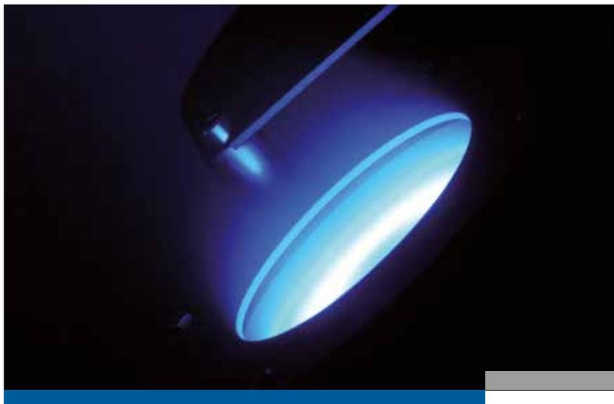
**TITANIUM:** The more titanium atoms that are ionized, the bluer the plasma inside the coating chamber looks.
