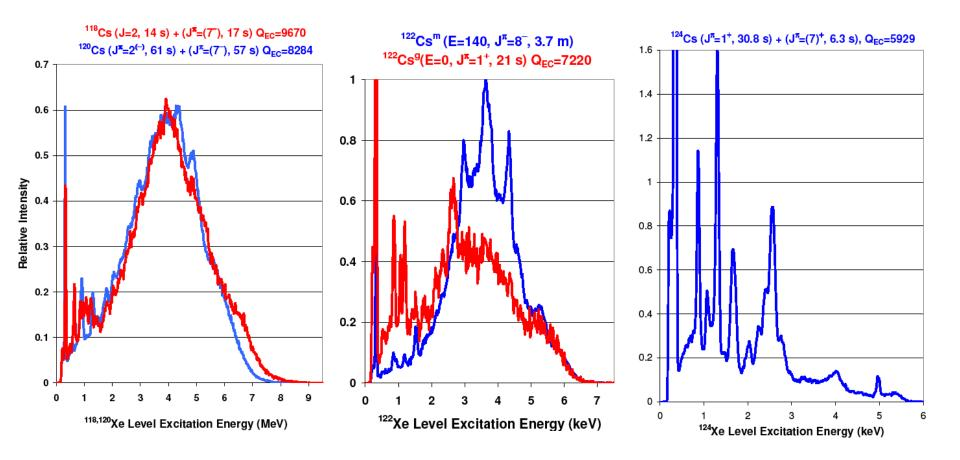
Typical spectra for <sup>118-124</sup>Cs decays. The TAS  $\gamma$ -ray spectra correspond to  $\beta$ -decay feeding intensities after correction for the detector response and EC/EC+ $\beta$ <sup>+</sup> ratio. Total detection efficiency ranged from 95% (0.3 MeV) to 55% (5 MeV).
