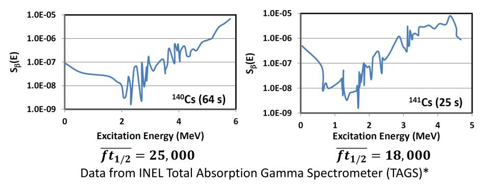
Experimental  $\beta$ -strengths do not peak within experimental energy window. These data would be incomplete templates for extrapolation to heavier Cs isotopes.
