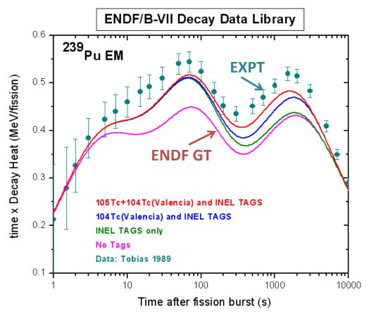
Decay heat calculations are dramatically improved by replacing ENDF Gross Theory based data with TAGS measurements from INEL (Greenwood *et al\**) and Valencia (Algora *et al\**). \* NIM A, 317 (1992) # J. Korean Phys. Soc. 59,1479 (2011).
