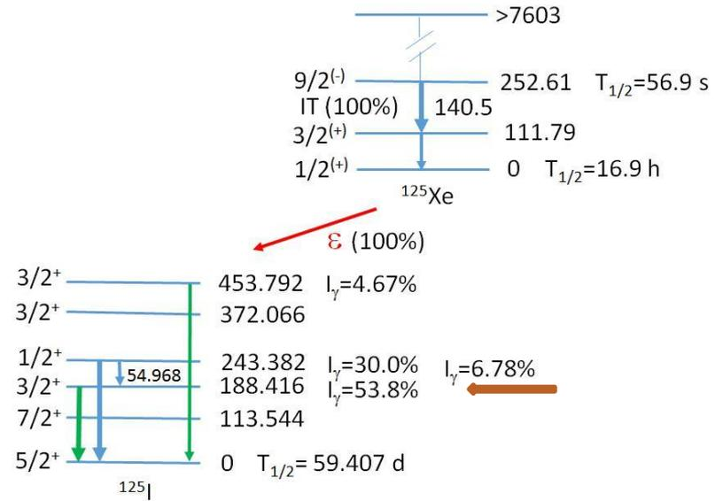
$E_{\gamma} = 188.4 \text{ keV}; I_{\gamma} = 53.8\%; T_{1/2} = 16.9 \text{ h}$
