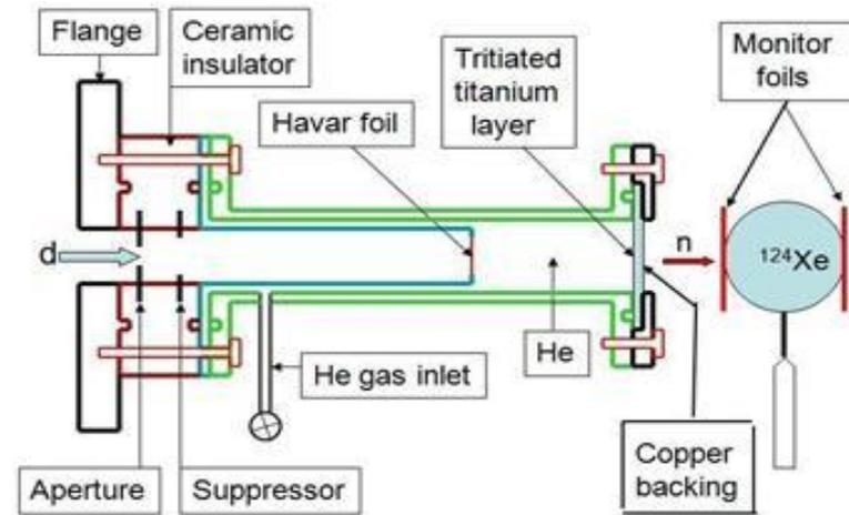
Schematic for (n,2n) measurements
