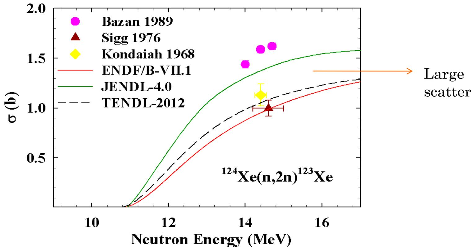
Obtaining new data is an important step to interpret the activation measurements at NIF
