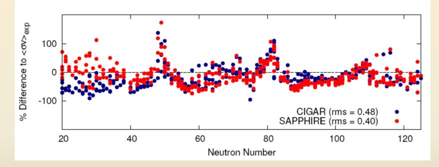
Identical nuclear models in both codes. Differences due to  $J\pi$  data truncation
