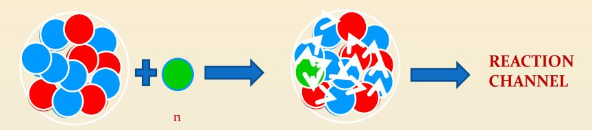
A Reaction takes place via intermediary C\* C\* must reach a state of thermodynamic eq.
