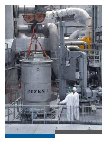
START: Loading of the new, fast reactor BN-800 at Beloyarsk. Photo: Rosenergoatom
