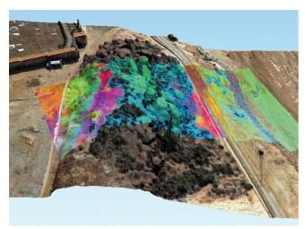
The HIF research team use drones and special cameras to locate and characterize ore deposits. This false-color hyperspectral image overlain on a 3D model reveals spectral contrasts of typical minerals associated with ore deposits in the Rio Tinto district in Spain. Picture credits: HZDR.
