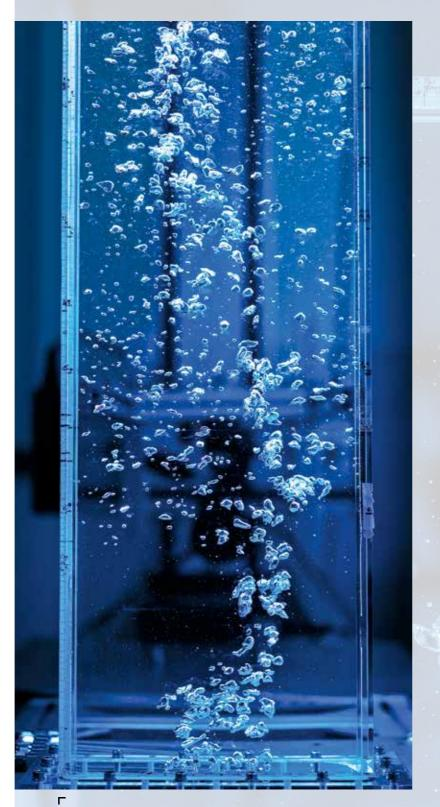
Unlike the reactors used in the chemical industry, the flow processes can be easily observed in transparent bubble columns. The similarity between the processes in both set-ups allows researchers to precisely investigate flow conditions. Source: A. Wirsig
