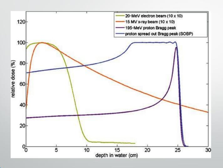
Figure 6: Depth-dose curve for electrons, Xrays and protons
