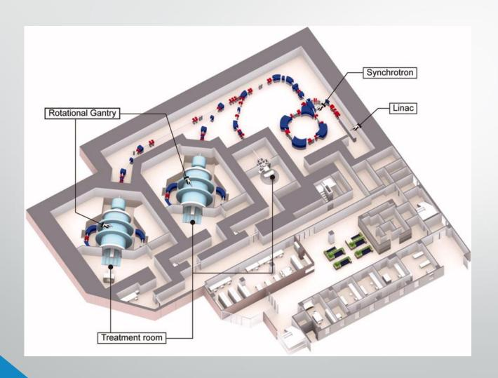
Figure 1: Layout of the Fukui Prefectural Hospital Proton Therapy Center
