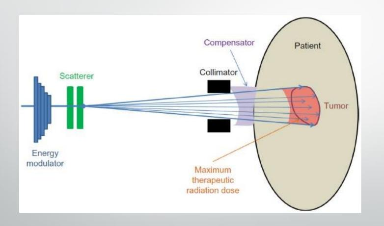
Figure 3: schematic structure of nozzle
