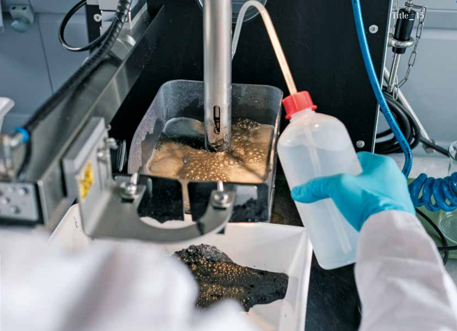
Froth flotation separates the valuable minerals from the gangue. Source: F. Schinski
