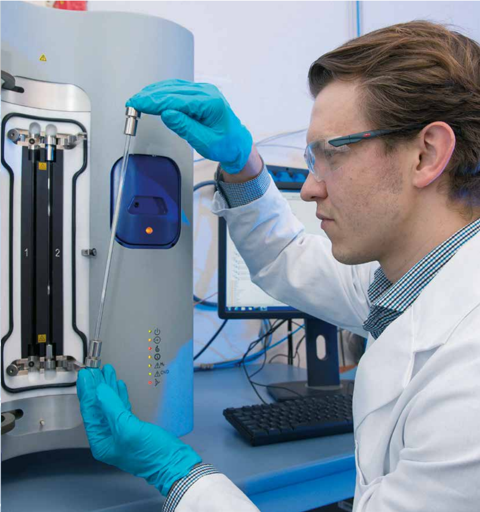
With a device known as an inverse gas chromatograph, Martin Rudolph can determine the surface properties of solids. Source: D. Müller
