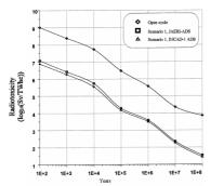
Radiotoxicity of transuranium elements in radioactive waste without (upper curve) and with reprocessing (lower ones). The radiotoxicity can be reduced by two orders of magnitude and thus the time of disposal is shortened by several 100 thousand years.
