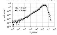
Neutron fluence entering the collimator (for each neutron bin, per electron started). [Graph taken from: J. Klug et al. "Development of a neutron time-offlight source at the ELBE accelerator", Nucl. Instr. Meth. A 577
