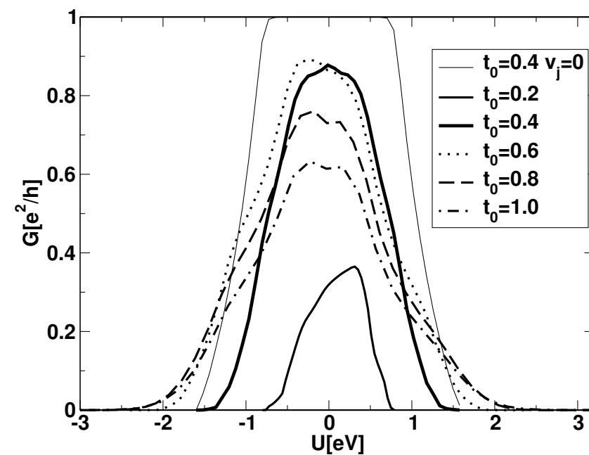
versus applied voltage bias for different hopping parameters from lead to thiophene,  $v_0 = 0$ ,  $v_j = -0.4$ , reference curve  $v_j = 0$
