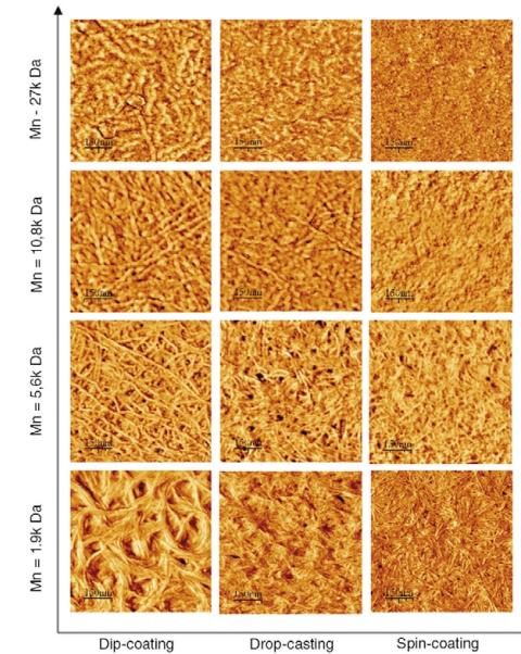
Tapping-mode AFM phase images obtained from P3HT fractions of different Mn and using different processing techniques
