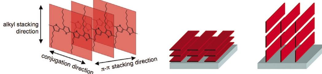
(a) Crystallite structure in polythiophenes. The conjugation direction and the p-p stacking direction are fast charge transport directions. (b) Plane-on (left panel) and edge-on (c) (right panel) texture of polymeric crystallites.
