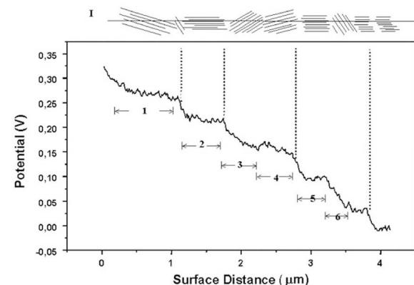
EFM measurement of the potential profile in a conducting polythiophene monolayer deposited between two electrodes
