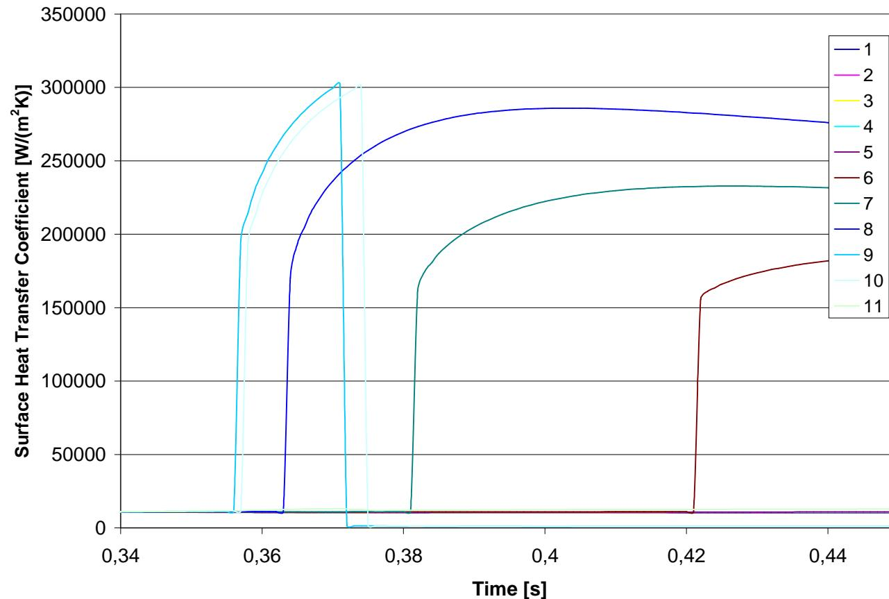
Switching between the different heat transfer regimes: convective heat transfer („Dittus-Boelter”), sub-cooled boiling („Thom”), transition boiling
