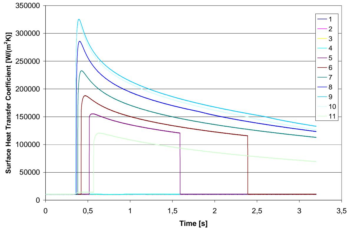
Switching between the different heat transfer regimes: convective heat transfer („Dittus-Boelter”), sub-cooled boiling („Thom”)
