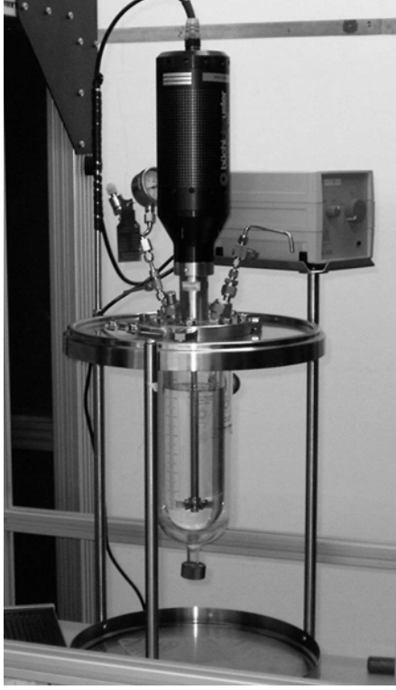
Fig. 2: Stirred tank reactor and stirrer geometry.
