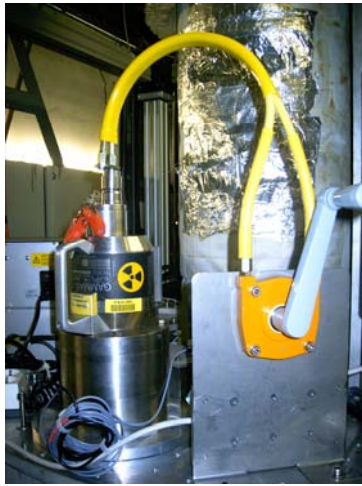
Fig. 4: View of the collimator with shielding container and Bowden cable.
