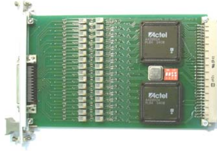
Fig. 2: Signal processing electronics (left) and view of one of the 10 pulse shaping and counting boards (right).
