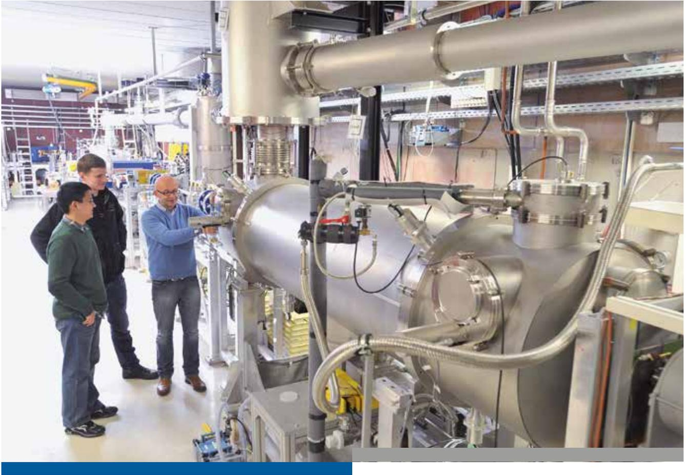
**THE HEART OF THE ELBE:** In an effort to enhance experimental options at the new Center for High-Power Radiation Sources, electron pulses from the electron accelerator that has been in operation for years have to be shortened and intensified by an entire order of magnitude. The electrons are used by the two free electron lasers, two new terahertz sources, as well as for the facilities for the generation of gamma and X-rays, positrons, and neutrons.
