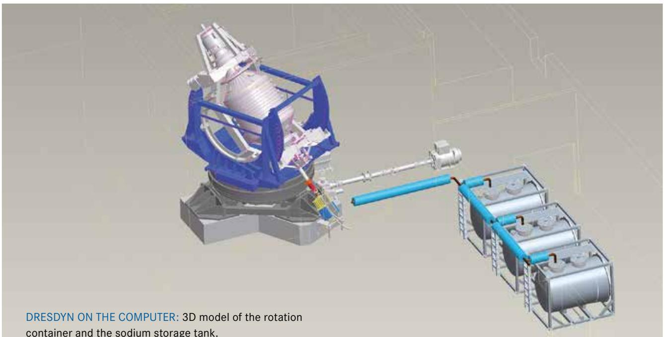
**DRESDYN ON THE COMPUTER:** 3D model of the rotation container and the sodium storage tank.
