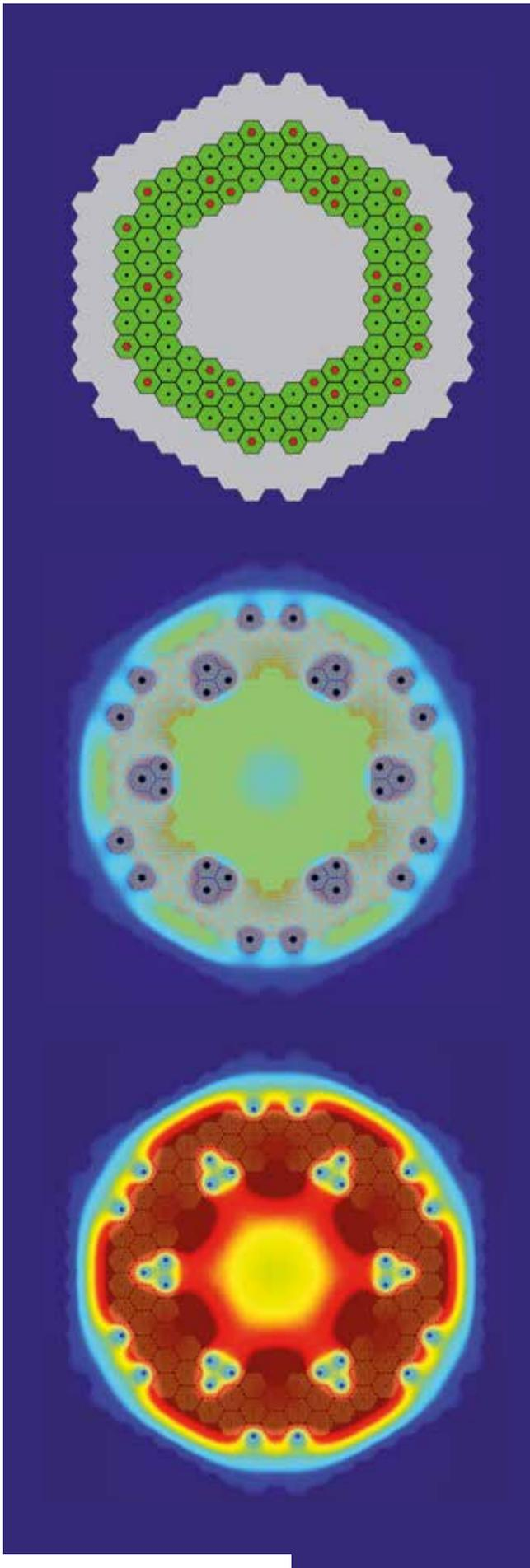
**FOCUSING ON GAS-, SODIUM-, AND LEAD-COOLED REACTORS:** The figure shows the results of the neutronic simulation of a high-temperature gas cooled reactor core using the SERPENT Monte-Carlo code. The upper figure presents the top view of the reactor core | *green - fuel blocks* | *red - control rods* | *grey - graphite reflector* |; the middle figure shows the thermal neutron flux distribution; the lower figure the total neutron collision rates distribution.
