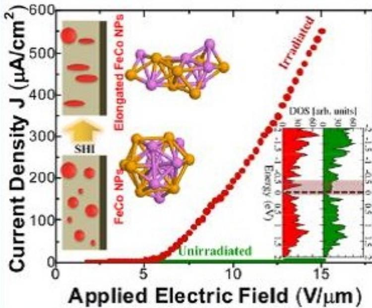
Figure 1: Shape engineering of FeCo nanoparticles embedded in SiO<sub>2</sub> matrix and Colossal rise in tunneling current
