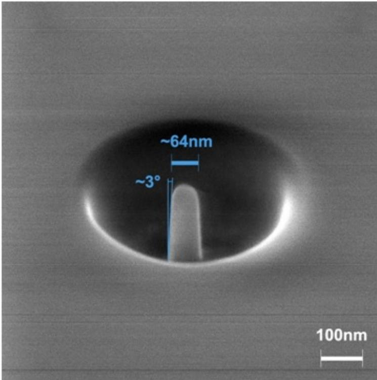
Figure 7: This nanopillar was produced by first milling with a  $\text{Ne}^+$  beam with alternating direction (outwards/inwards), and then by polishing with a  $\text{He}^+$  beam directed only inwards.
