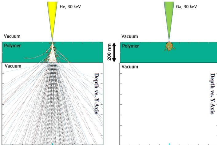
Figure 1: SRIM simulation of typical beam interaction for light ions (He) versus heavy ions (Ga) for an unsupported polymer film of 200 nm thickness. Field of view is 1  $\mu\text{m}$ .
