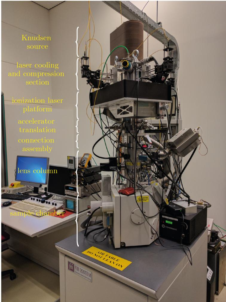
Figure 4: Rb<sup>+</sup> FIB installed at CQT Labs
