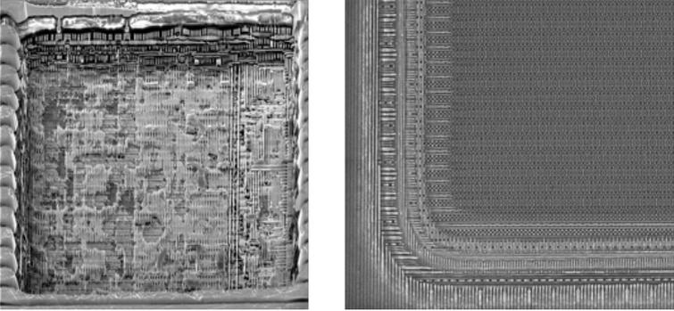
Figure 3: Delayering attempted without gas (left) and same process using new chemistry (right)
