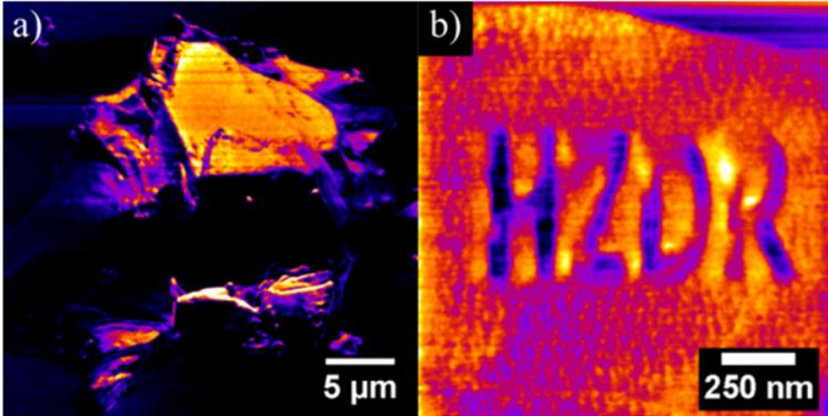
Figure 2: (a) SIMS+ image of a rock salt crystal on SiO<sub>2</sub>. (b) SIMS+ image of the Ne ion beam milled letters HZDR. The contrast arises as the NaCl has been partially removed by the Ne milling.
