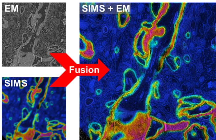
Figure 4: Image fusion in the EM/SIMS context. Top left: HR-SEM of a stained mouse brain tissue sample; bottom left: SIMS map of the  $^{15}\text{N}$ -enrichment after an isotope uptake experiment. Right: Result of Laplace pyramid image fusion of EM and SIMS data. This fused image allows for reliable identification of cellular features while retaining the spectroscopic information of the SIMS data set.
