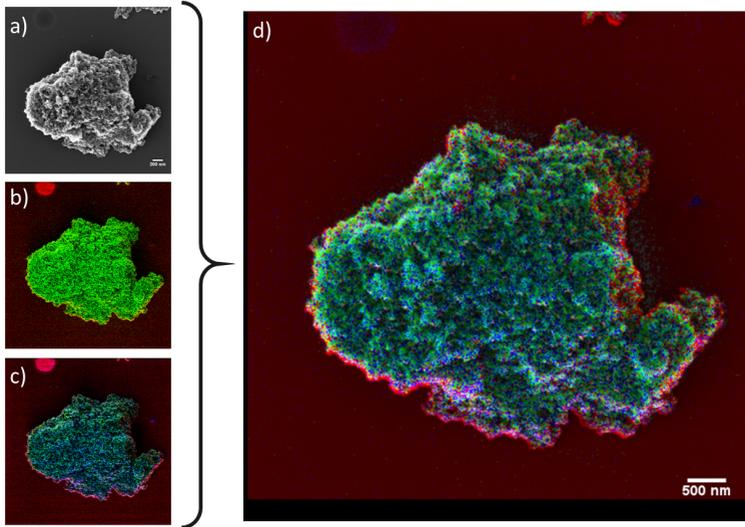
Figure 3: Analysis of Ti nanoparticles deposited on InP substrate. a) SE image (20 keV He beam, 1024x1024). b) and c) SIMS images of Na (blue), Ti (green) and In (red) (20 keV Ne beam, 2 pA, 2 ms/pixel, 512x512). d) Combined SIMS and SE imaging according to the methodology presented in [6]. Scale bar 500 nm.
