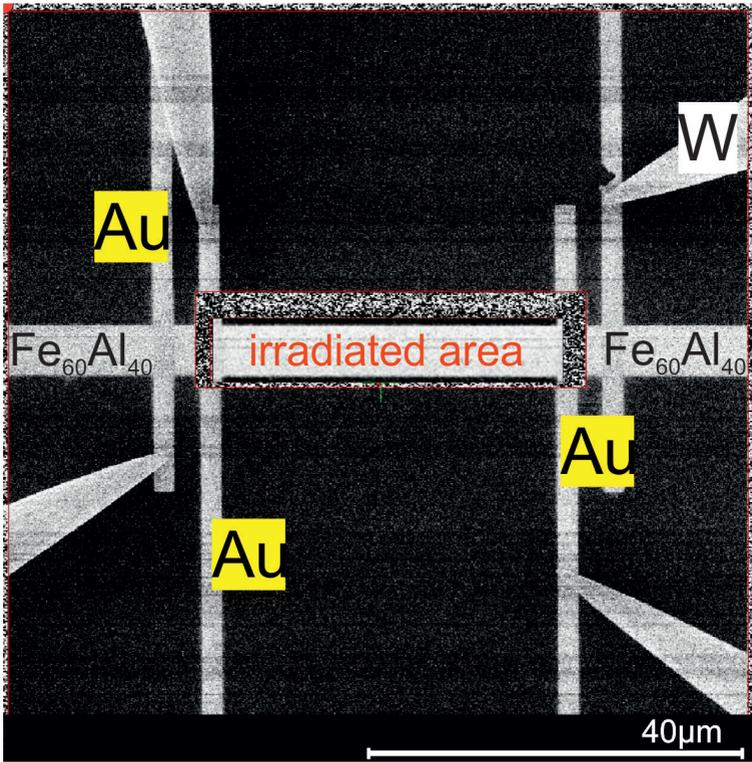
Figure 6: Fe<sub>60</sub>Al<sub>40</sub> wire with gold contact lines, contacted with tungsten probes. The region of Ne<sup>+</sup> irradiation is marked.
