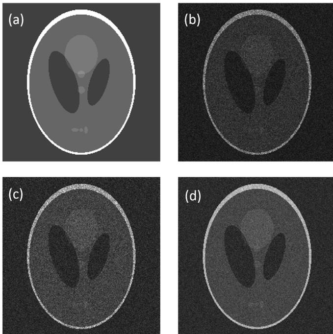
Figure 6: Simulated HIM experiment for a sample with mean secondary electron yield in  $[2, 8]$ : (a) Ground truth image with secondary electron yield rescaled from 2 to 8. (b) Conventional HIM image with MSE of 0.5934. (c) Maximum likelihood estimation with MSE of 0.5513. (d) Our work without dose reduction with MSE of 0.2297. These results have not utilized spatial regularization.
