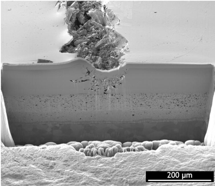
Figure 7: Site specific cross-sections for scratch testing and adhesion in paint coatings.
