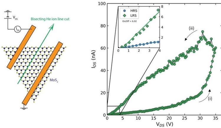
Figure 4: Left: Schematic of fabricated device. Right: Typical IV sweep showing switching from high to low resistance states.
