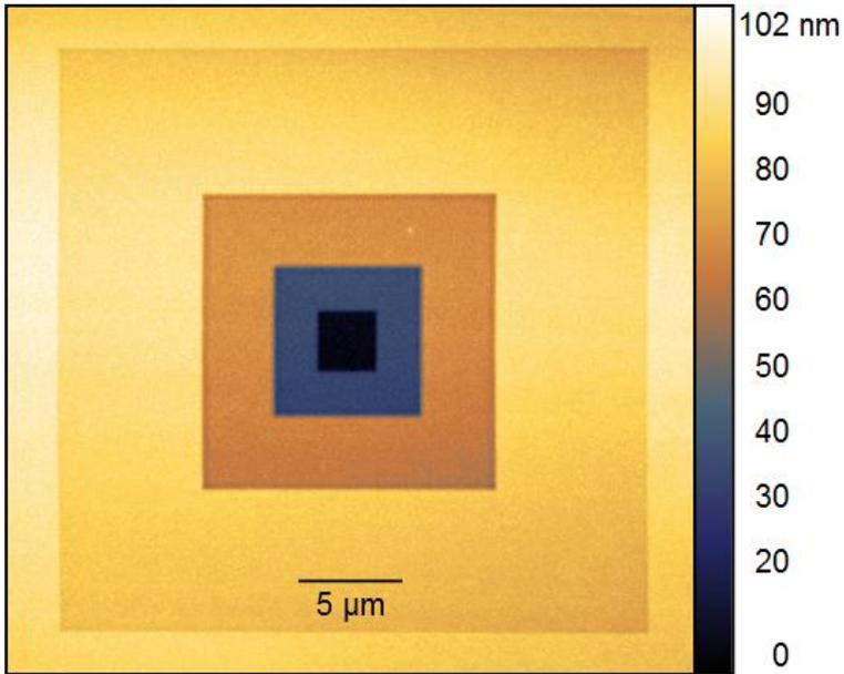
Figure 2: Atomic force microscope image of a microstructure fabricated in Au-Pd/PMMA system with a Helium FIB in a Zeiss Nanofab HIM.
