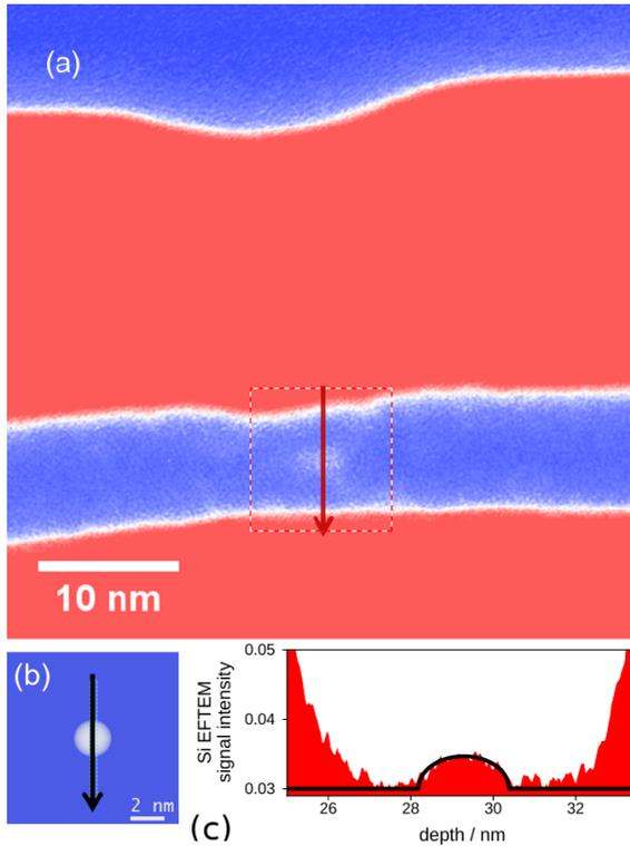
Figure 2: (a) EFTEM shows 17eV Si plasmon-loss signal, compared to (b) modulated dot signal the formation of single Si ND via HIM Ne<sup>+</sup> implantation is confirmed (c)
