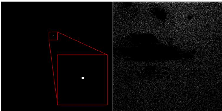
Figure 5: Transmission HIM images taken (left) without a sample and the beam focussed on the camera resulting in just one pixel registering counts, and (right) with a thin Au sample in place showing strong scattering. Dark areas with no counts are due to dead pixels.
