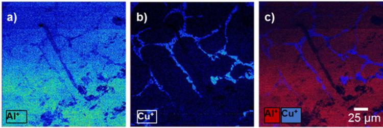
Figure 6: ZEISS ORION NanoFab SIMS generated elemental mapping distribution of Al (a) and Cu (b) on CuAl alloy sample. Image (c) represents a composite image. Field of view is 225µm.
