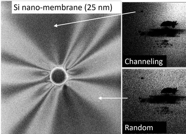
Figure 4: Example of channeling through a 25 nm Si nano-membrane. HIM secondary electron image with transmission images from areas indicated. Grey regions better aligned, more channeling. White areas higher SE intensity less channeling.
