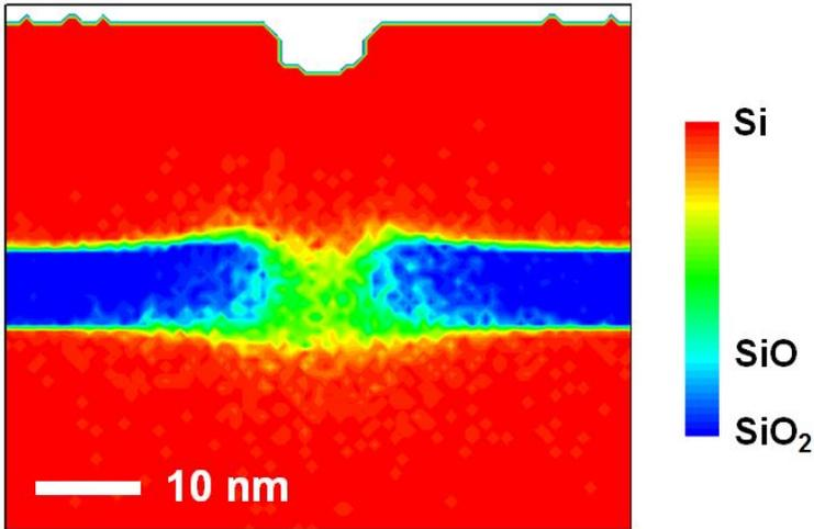
Figure 1: Atomic mixing and surface erosion in a Si (20 nm) / SiO<sub>2</sub> (7 nm) / Si layer stack after irradiation with 30.000 Ne ions at an energy of 25 keV, a Gaussian beam profile of 5 nm FWHM, and a scan area of 3x3 nm<sup>2</sup>, as obtained from TRI3DYN 3D dynamic computer simulation. The graph shows the local composition as quantified by the color code, averaged over a central slice of 1.33 nm thickness.
