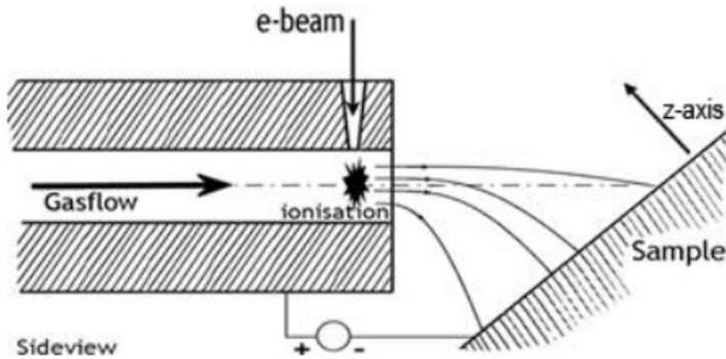
Figure 5: Illustration of the ionization process and the attraction of positively charged ions towards the surface.[1]
