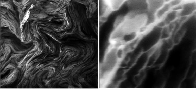
Figure 5: Carbon graphite: Example of images obtained with ColdFIB at 30 keV, with a different field of view, respectively 10 and 1  $\mu\text{m}$ .
