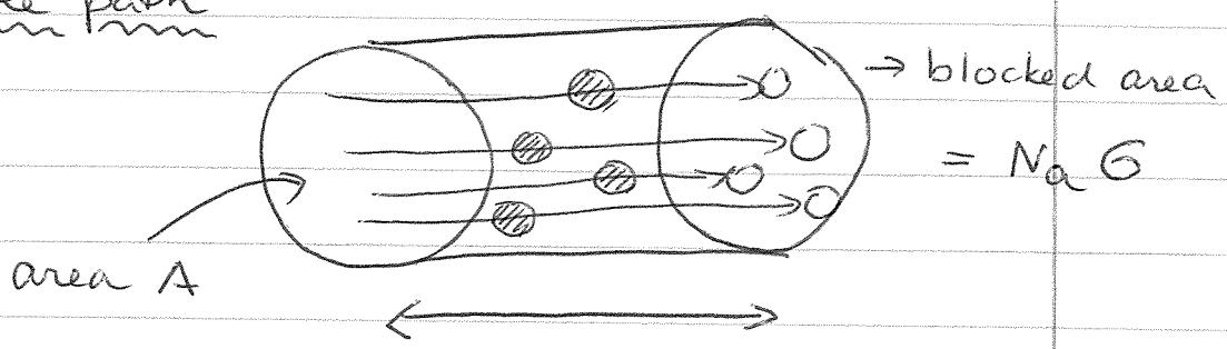
$\rightarrow$  differential probability for a collision:  $d\omega = \frac{N_A G}{A} = n_a G \sigma z$
