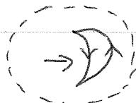
$\rightarrow$  each collision moves particle by 1 banana orbit
