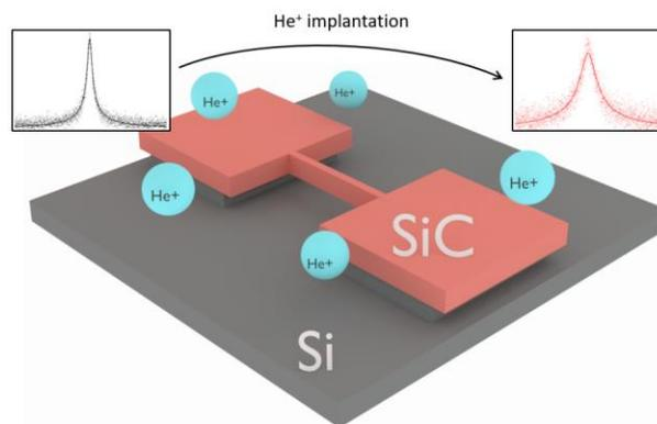
Figure 1: He<sup>+</sup> implantation on resonators in 3C-SiC [Insets show change in the resonance spectrum]
