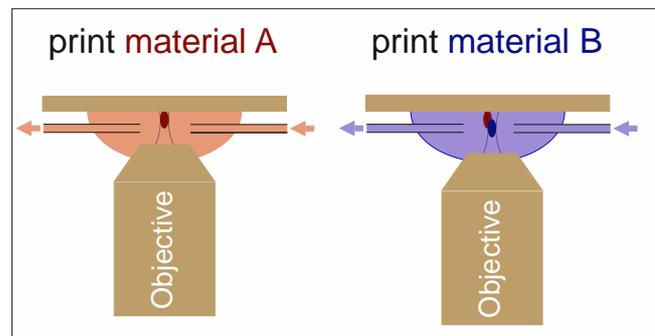
**Figure 1b:** Schematic of in situ material replacement for efficient high-resolution functional 3D micro-printing based on 2-photon polymerization based 3D laser writing.
