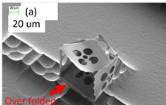
**Figure 1a:** SEM images of typical results in the current process state of design optimization for dry releasing Al<sub>2</sub>O<sub>3</sub> structures from a silicon carrier.
