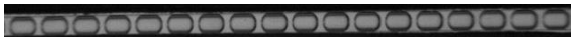
Figure 4. Taylor flow of isobutane – nitrogen with 2.157 ml/min nitrogen (1.783E-03 m/s) and 826 mg/h Isobutane (5.284E-04 m/s) at a pressure of 35 bar and 25 °C.
