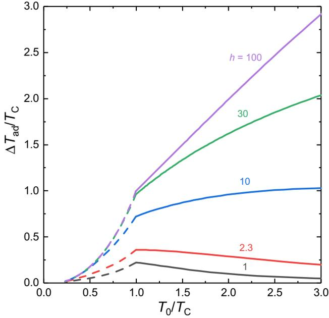
FIG. 1. Calculated reduced adiabatic temperature change of Gd as a function of the reduced initial temperature for different values of the dimensionless magnetic field  $h$ , defined in Eq. (12). The dependence for  $T_0 < T_C$  (dashed curves) is complex to derive and is not considered in this work.
