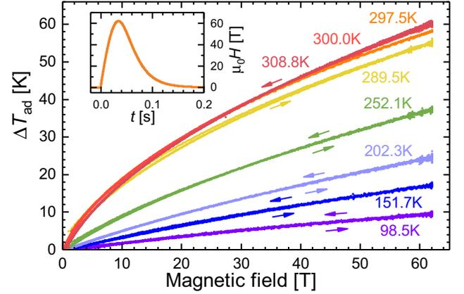
FIG. 2. Adiabatic temperature change  $\Delta T_{\text{ad}}$  of a gadolinium single crystal in pulsed magnetic fields up to 62 T at different initial temperatures  $T_0$ . For all curves, both the magnetization and the demagnetization branches are plotted. Experimental data presented in this and other figures are measured with the magnetic field vector along the (0001) direction. The inset shows the temporal profile of the magnetic field pulse. The rise time amounts to 33 ms.
