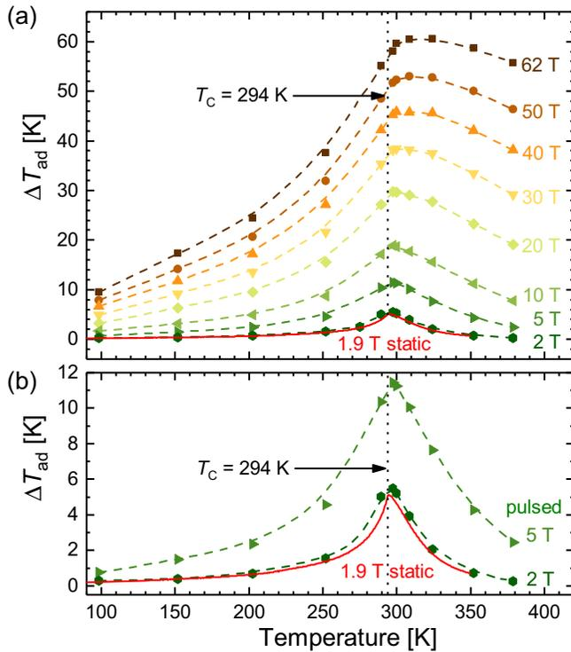
FIG. 3. (a) Adiabatic temperature change  $\Delta T_{\text{ad}}$  as a function of temperature for different magnetic fields. The data points were extracted from the magnetic-field dependencies of  $\Delta T_{\text{ad}}$  for given field values. They are connected with dashed lines as a guide to the eye. The solid line shows the data obtained from direct measurements of the adiabatic temperature change under quasistatic conditions. (b) The low-field region of (a).
