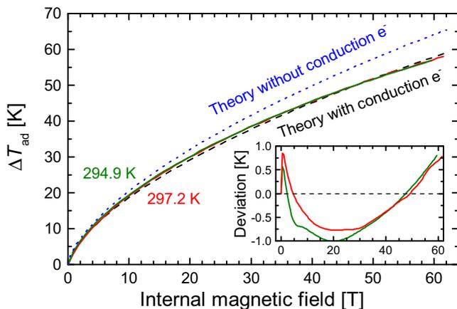
FIG. 5. Comparison of the adiabatic temperature change at two different starting temperatures near  $T_C$  and the theoretical curve with and without contribution of the conduction electrons to the heat capacity (dashed and dotted curves). The inset shows the difference between the theoretical and the experimental curves.
