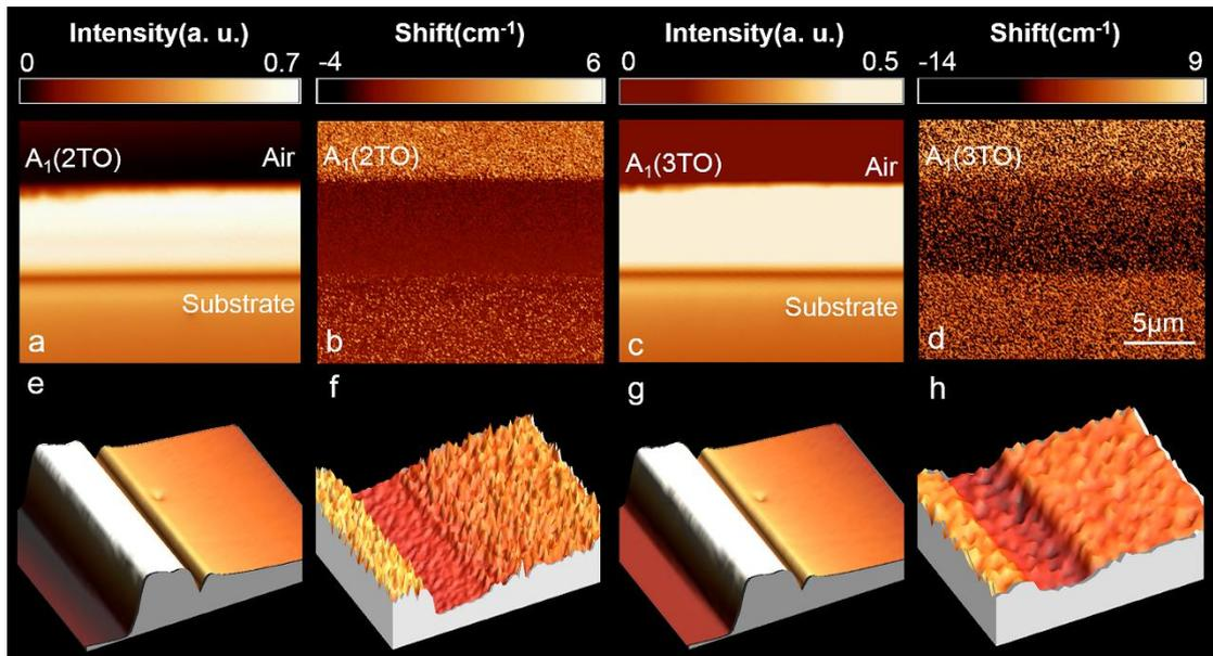
**Figure 7.** 2D spatial distributions of (a) intensity and (b) shift of the  $A_1(2TO)$  mode around  $207\ \text{cm}^{-1}$ , and spatial distributions of (c) intensity and (d) shift of the  $A_1(3TO)$  mode around  $565\ \text{cm}^{-1}$  obtained from the end-face of the  $15\ \text{MeV}$  swift  $O^{5+}$  ion irradiated KTN sample at room temperature, respectively, (e)-(h) correspond to the
