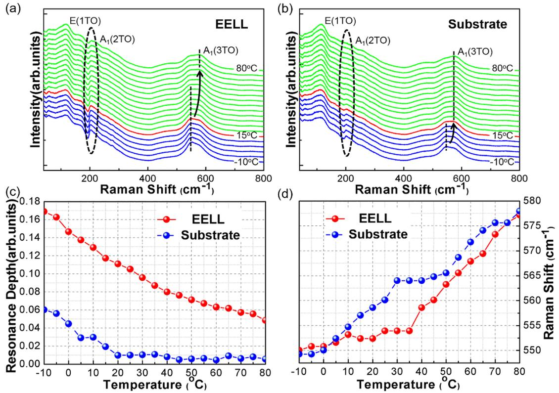
**Figure 3.** Raman spectra at different temperatures with an interval of 5  $^{\circ}\text{C}$  for (a) the EELL at a depth of  $\sim 3 \mu\text{m}$  beneath the surface and (b) the substrate of the 15 MeV swift  $\text{O}^{5+}$  ion irradiated KTN crystal. The temperature dependence of (c) the resonance depths of the  $A_1(2\text{TO})$  mode and (d) the peak positions of the  $A_1(3\text{TO})$  mode obtained from the EELL and the substrate of the irradiated KTN sample, respectively.
