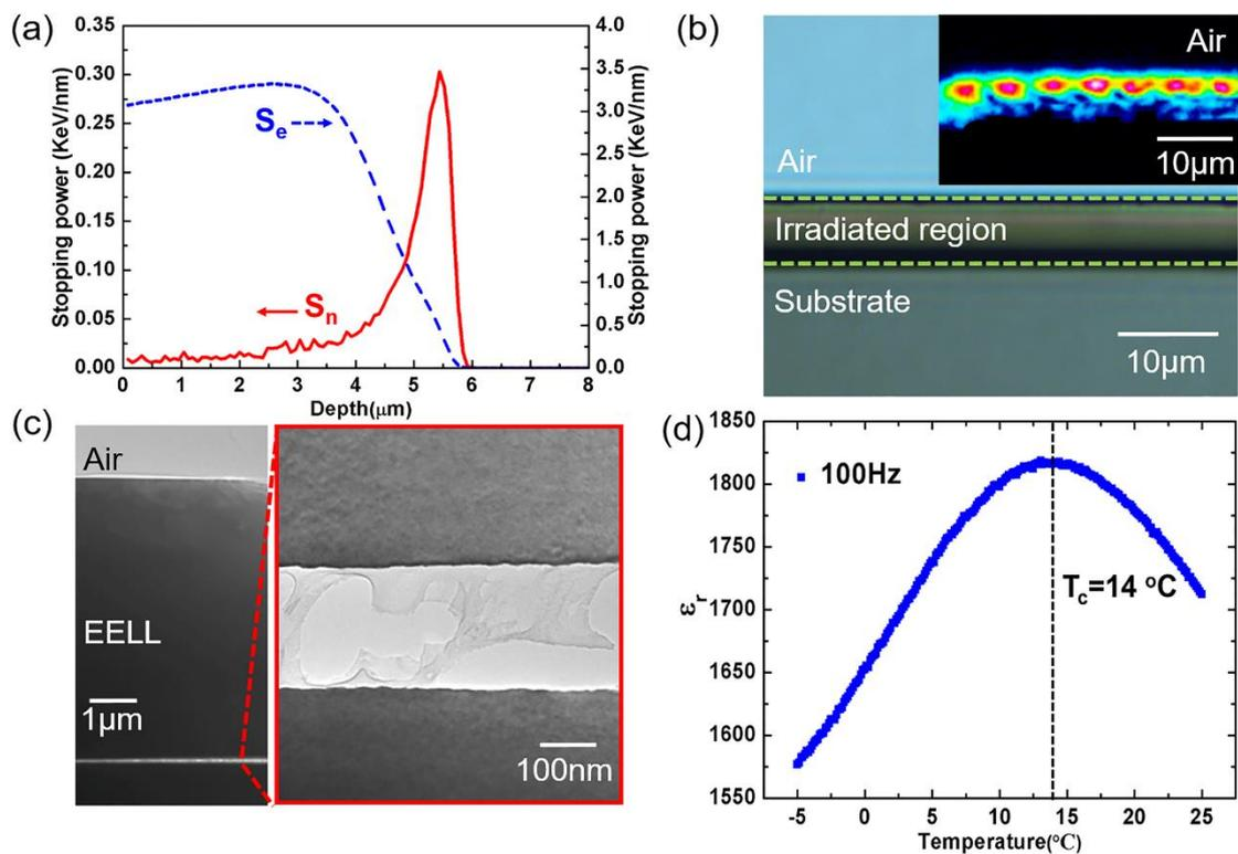
**Figure 1.** (a) The electronic (blue dash line) and nuclear (red solid line) stopping power profiles of the 15 MeV swift  $\text{O}^{5+}$  ion irradiated KTN crystal as a function of penetration depth from the sample surface, respectively, (b) the cross-sectional microscope image of the swift  $\text{O}^{5+}$  ion irradiated KTN crystal, and the inset shows the
