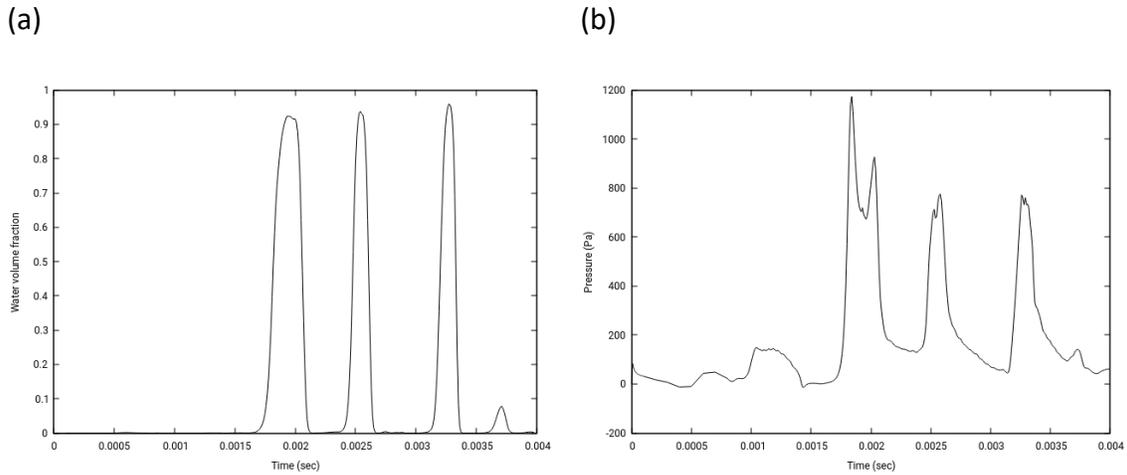
Figure 4. Spot values of (a) water volume fraction,  $\alpha_w$ , and (b) pressure,  $p$  (Pa) as a function of time, at point P, located in the centre of the gas channel midway between the PTL specimen and the gas outlet.
