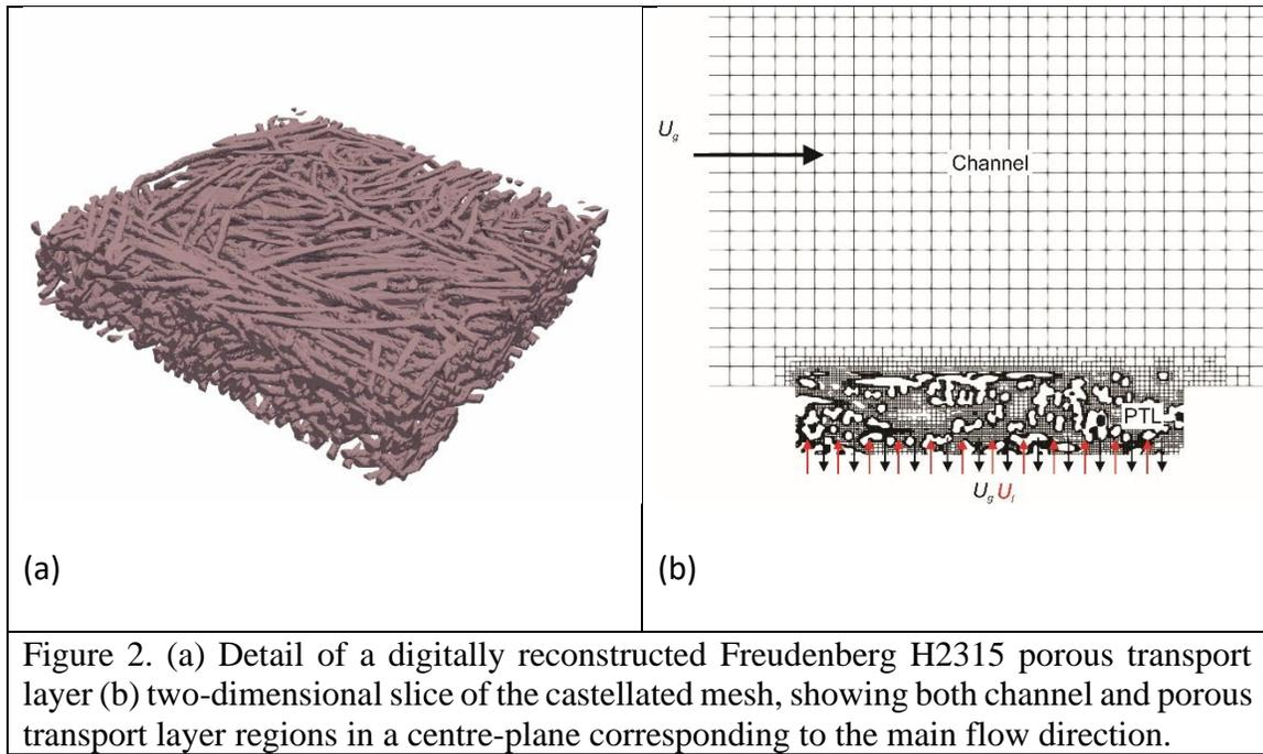
Figure 2. (a) Detail of a digitally reconstructed Freudenberg H2315 porous transport layer (b) two-dimensional slice of the castellated mesh, showing both channel and porous transport layer regions in a centre-plane corresponding to the main flow direction.
