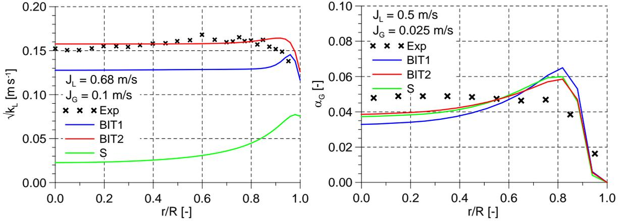
Fig. 1: Comparison of different BIT models (BIT 1 - Rzehak & Krepper, 2013b; BIT 2 Ma et al., 2017; S - Sato et al., 1981) a) Measured and calculated turbulent kinetic energy for the experiment by Shawkat et al. (2008), b) Measured and calculated gas volume fraction for the experiment of Hosokawa et al. (2007)
