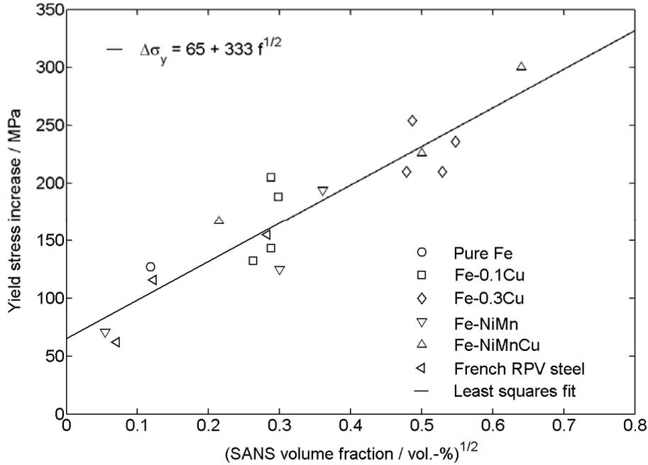
Fig. 3: Scatterplot of yield stress increase and square root of volume fraction [5]
