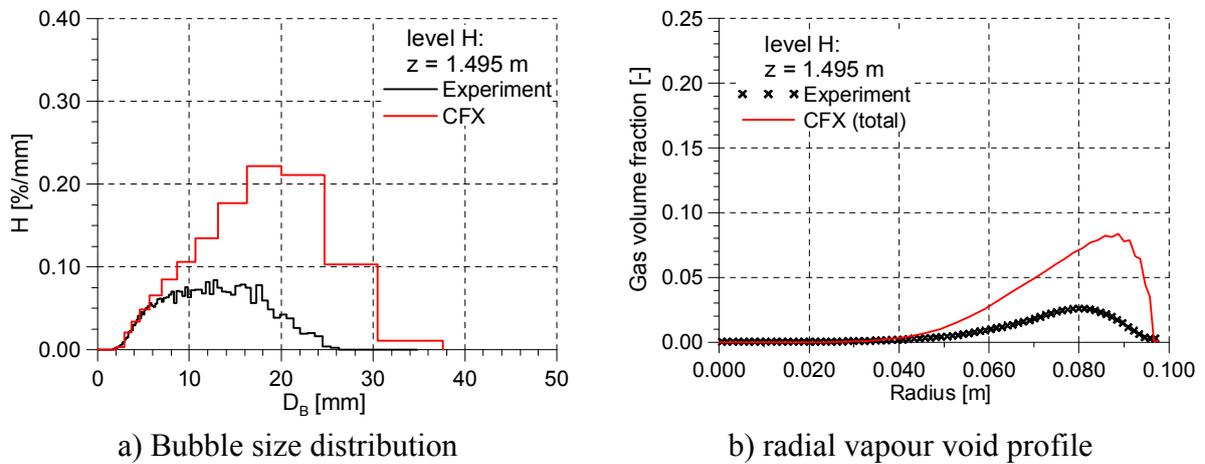
Fig. 3: Development of the vapour void at different distances  $z$  from the steam injection
