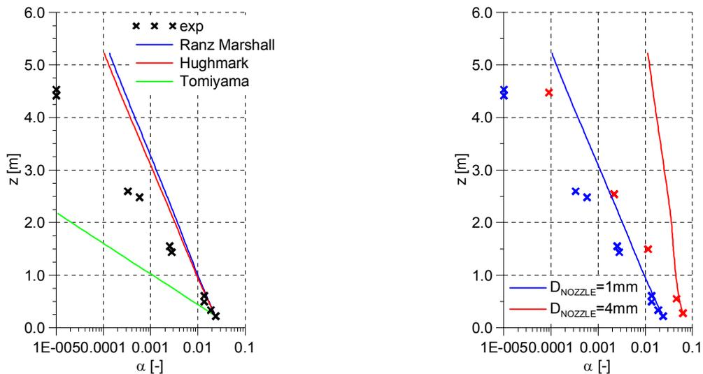
a) Influence of the heat transfer model, (Nozzle diameter:  $D_{\text{Nozzle}}=1\text{mm}$ )
