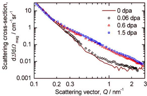
Fig. 5: Magnetic scattering cross sections for Fe-9Cr
