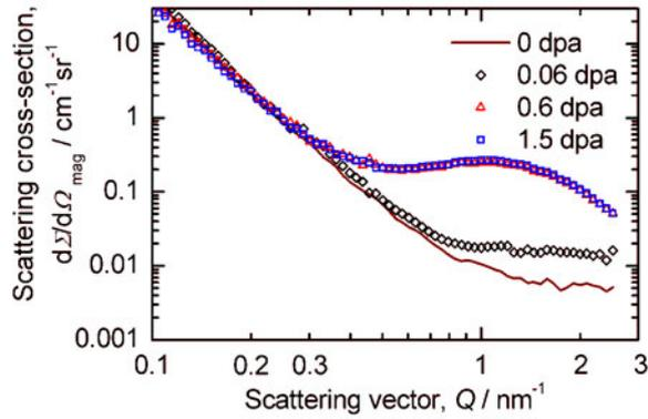
Fig. 7: Magnetic scattering cross sections for Fe-12.5Cr
