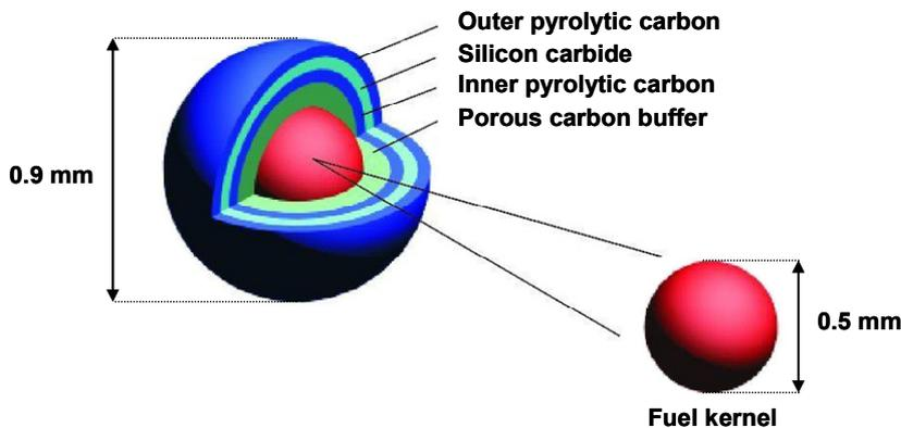
Fig. 1: TRISO coated fuel particle
