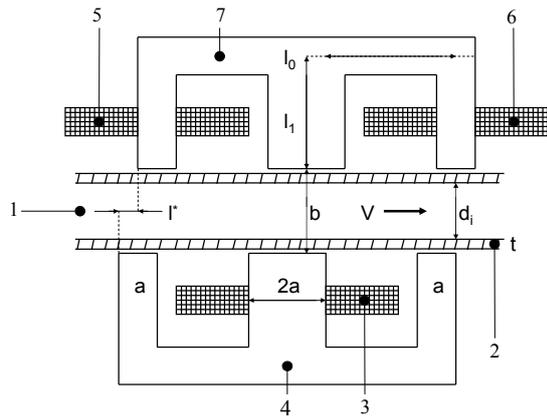
Fig. 1b: Sketch of the phase-shift flow meter in the asymmetric adjustment. 1-duct, 2-duct-wall, 3-emitter coil, 4,7-laminated magnetic iron, 5,6-receiver coils,  $l^*$ -displacement length between emitter and receiver coils
