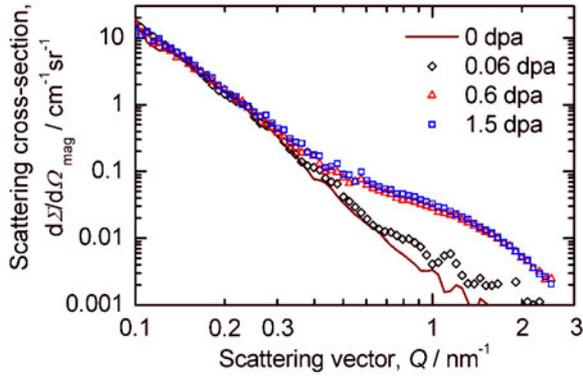
Fig. 1: Magnetic scattering cross sections for Fe-2.5Cr
