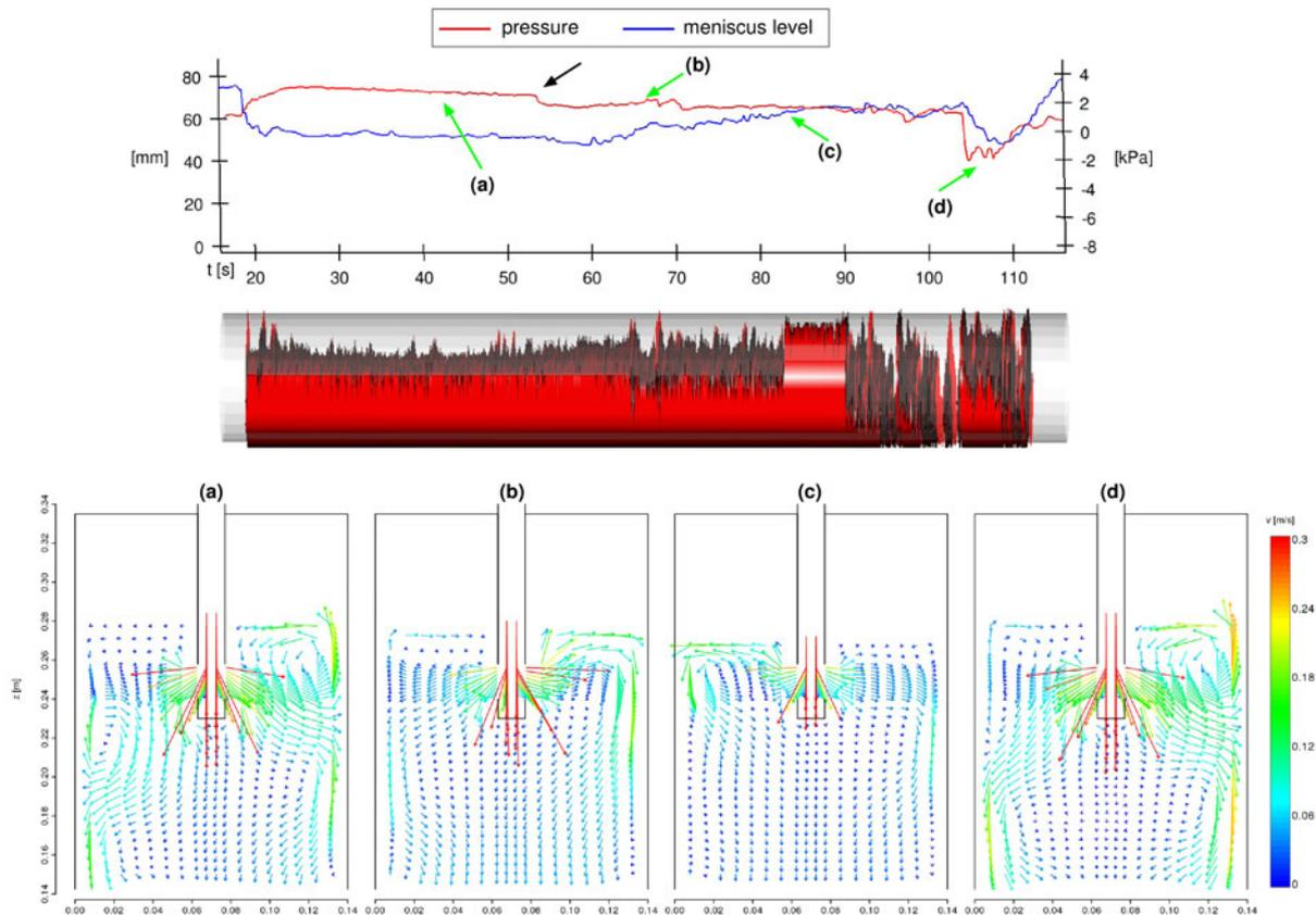
Fig. 4: Reconstructed gas/liquid metal distribution by the MIT sensor for the experiment with  $500 \text{ cm}^3/\text{min}$  Argon flow. Additionally the velocity field reconstructed by CIFT is given for four different instants in time
