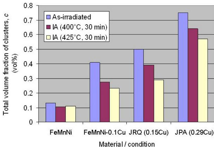
Fig. 4: Effect of post-irradiation annealing on volume fraction of scatterers
