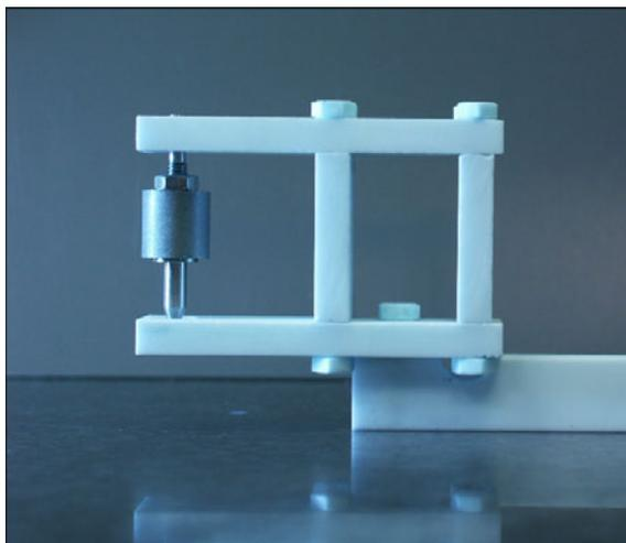
Fig. 2a: Single-magnet rotary flow meter
