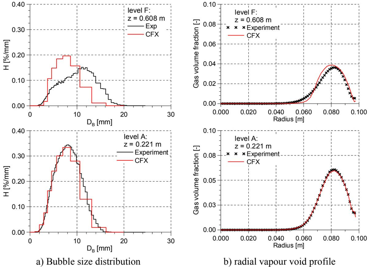
Fig. 2: Development of the vapour void at different distances  $z$  from the steam injection
