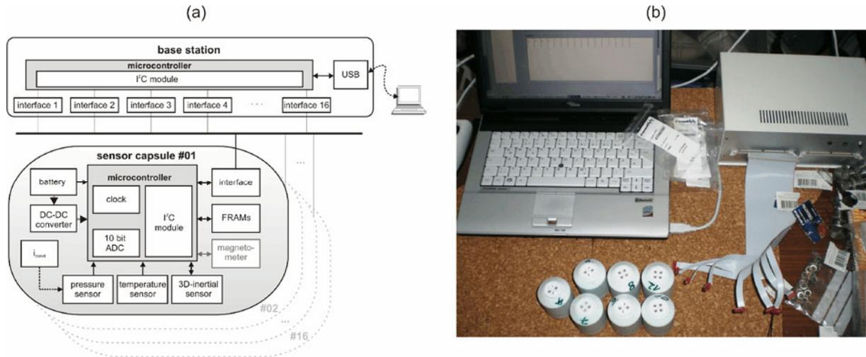
*Fig. 1: Block diagram of the base station with 16 individual connections and the autonomous sensor particle's electronics (a) and photograph of the measurement system used during the trials, comprising a PC, the base station with cable connections and 7 fabricated sensor particles (b)*
