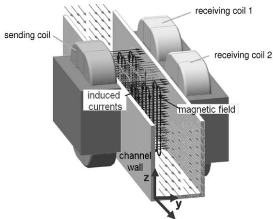
Fig. 1a: Set-up of the phase-shift flow meter
