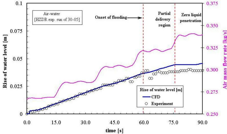
Fig. 4: Example of the calculated the rise of the water level inside RPV channel
