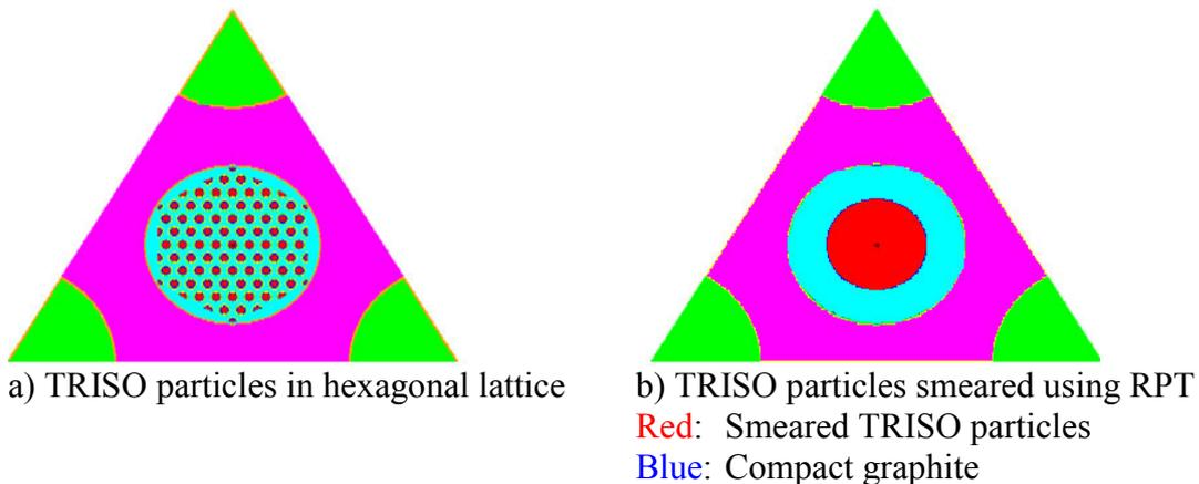
Fig. 4: Prismatic fuel lattice models
