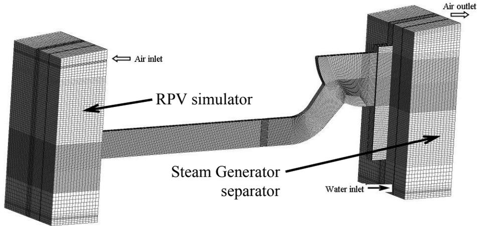
Fig. 1: Calculation meshes
